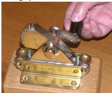
Jamming Cleat for continuous jib sheet
