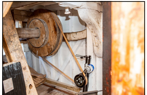
Connecting old and new: The belt drive that the Tide Mill uses to power its new micro generator.
