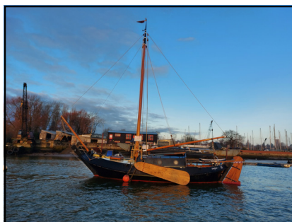
Dulcibella , a Dutch 'schokker' (pleasure boat) has recently undergone extensive refurbishment carried out largely by the Woodbridge Boatyard apprentices. Notice her new leeboard, made of best quality oak (from France).
