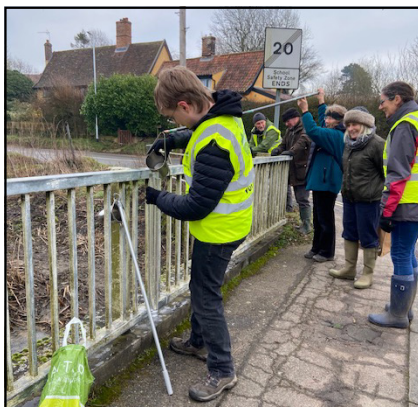
Debenham Green Team volunteers measuring 'turbidity'. By looking down a Perspex tube the cloudiness of the water can be measured—this will indicate the amount of particles hazardous to fish and other wildlife. The samples are then tested to determine the types of particles.
